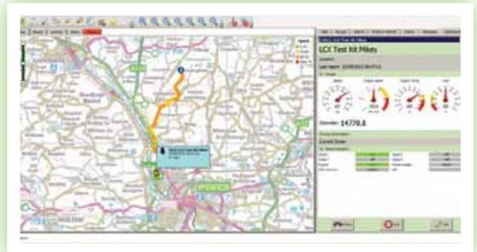
**Driver Behaviour,** with locutu you can get real time driver behaviour , with a single click you can view engine rev's, fuel guage, throttle position, engine temperature and engine load.
